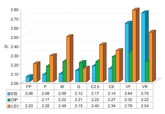
With three different methods it is possible to obtain comparable results for the fractal dimension  $D_F$ . LSV measurements provide too high values for smooth surfaces. Here a disturbing influence of the passive layer must be taken into account. In contrast to electrochemical methods (integral methods) for DIP only a small fraction of the surface is analysed. This could be a reason for too small values obtained for rough surfaces by DIP.
