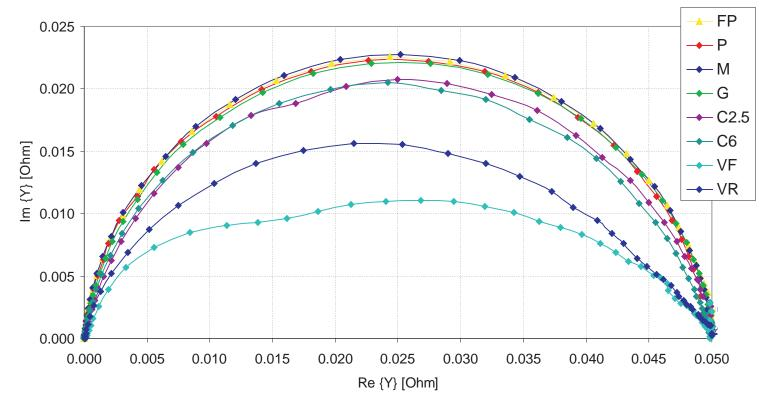
Semicircles representing the admittance are depressed with increasing roughness.
